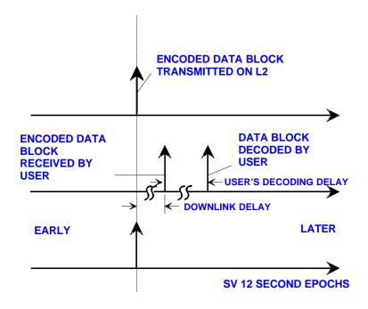
Figure 3-16. Convolutional Transmit/Decoding Timing Relationships
