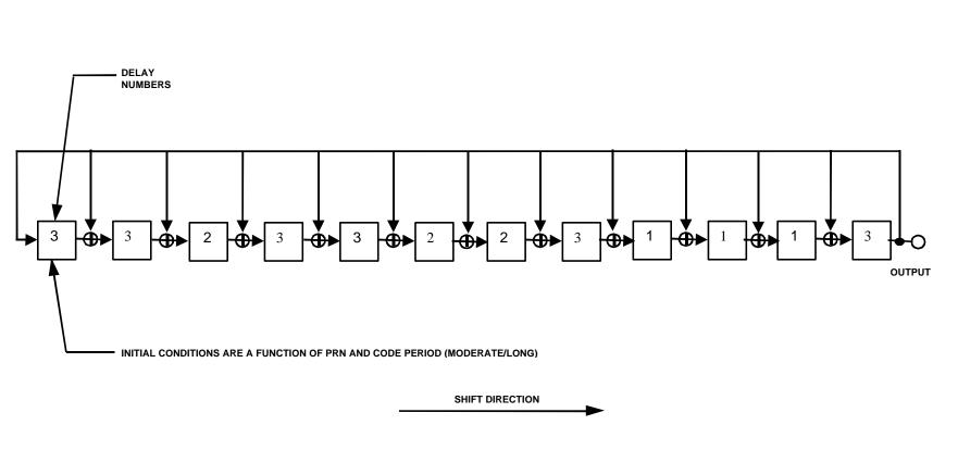
3-14 L2CM/L2CL Shift Register Generator Configuration
